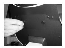
Use coin to remove battery access panel.
