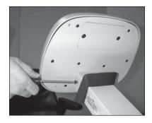
Remove three screws. (Hold onto display so it does not fall!)
