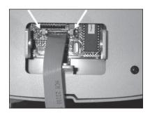
Release 2 locking tabs on each side of connector.
