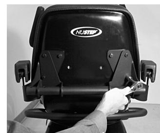
3. Remove one old shorter screw and install one 51041 storage hook using new longer 51042 screw. Repeat. Don't over tighten screws.
