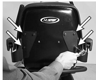
2. Position 51014 seat mount bracket over armrest brackets, start four 51039 flange cap screws and tighten to 200 +/- 20 inlbs. (23 +/- 2 Nm)
