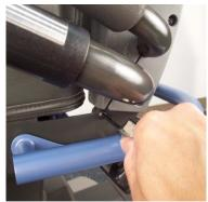
Slip 50395 guide bracket through slot between seat cushion and bracket on left side of seat.
