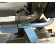
Slip 51600 bracket through slot between seat cushion and bracket on right side of seat. Install two 51756 screws with 51757 washers using 5mm hex key. Tighten screws
