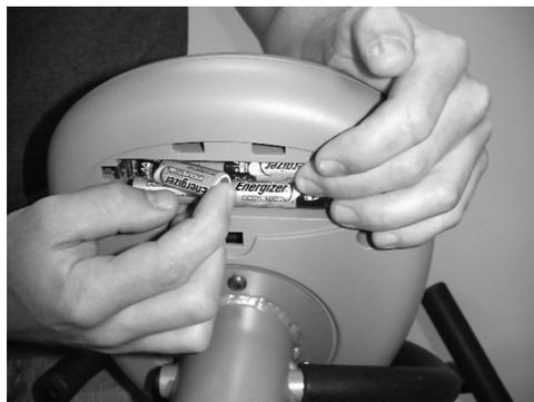
*Note: Ensure batteries are properly installed in the correct direction as indicated by battery and polarity symbols in console battery case.*
