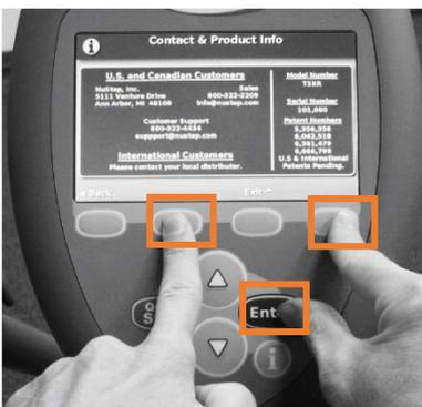
4. On the *Manager Mode* screen, use the down arrow to scroll to *Change Factory Defaults* screen and press Enter
