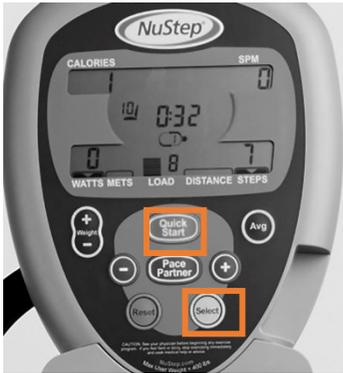
2. On any *Manager Mode* screen. Press the *Quick Start* and the *Avg* buttons at the same time to toggle BLE off and on.
