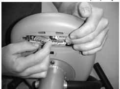
in the correct direction as indicated by battery and polarity symbols in console battery case.
