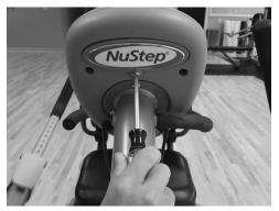
2. Replace the 4 AA alkaline batteries. (NiMH rechargeble batteries may also be used.) Note: Ensure batteries are properly installed
